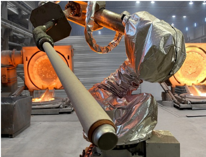
PolySAMPLE: Sampling robotic solution for foundries
