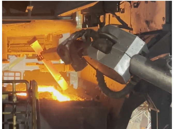
PolyCAST: Multitool robotic solution for caster operations
