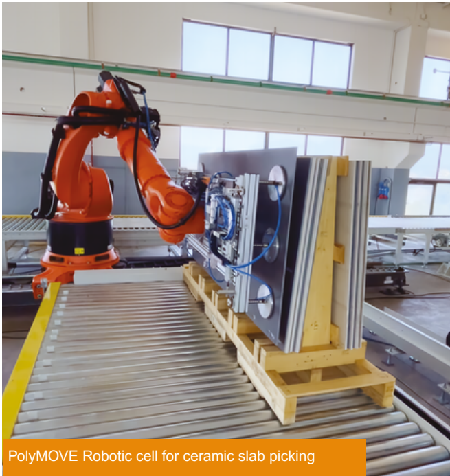
PolyMOVE Robotic cell for ceramic tile handling
